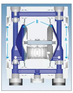
AODD pumps offer superior containment due to the fact that they don't use mechanical seals and packing. In the Almatec pump illustration shown above, the stainless steel Containment Ring (A) clamps tightly on two sides of the pump housing, pulling it together over the smooth, integrated metal core diaphragm (B), which further increases safety and ensures a tight seal.
