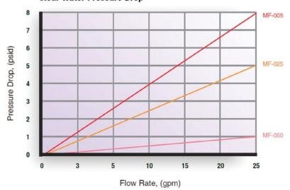
This chart show the Vorex® filter cartridge pressure drop as related to flow-rate per 10 inch cartridge length. Results may vary in actual service.
