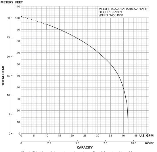
= A 1<sup>1</sup>/4" minimum discharge pipe requires a minimum flow of 10 gpm to maintain a 2 ft./sec. scouring velocity. Flows less than 10 gpm will allow solids to settle in the pipe.
