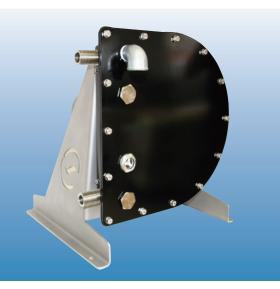
Applications from Fish Processing to Luce Slurry Transfer Enviroflex L Series pumps provide all the benefits of other peristaltic pumps, with a number of key benefits — slower operating speed for a given flow rate; and rotating rollers for soft hose compression. This provides a longer hose life and reduced power consumption.
