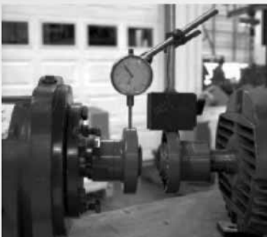
FIGURE 10 DIAL INDICATOR SETUP
