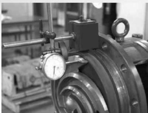
FIGURE 25 IMPELLER RUNOUT CHECK
