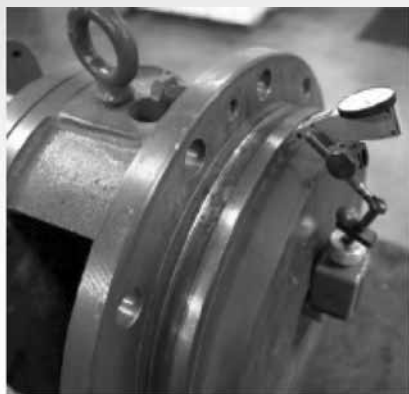
FIGURE 24 STUFFING BOX COVER RUNOUT CHECK
