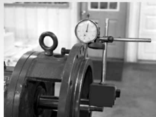
FIGURE 23 ADAPTER FACE RUNOUT CHECK
