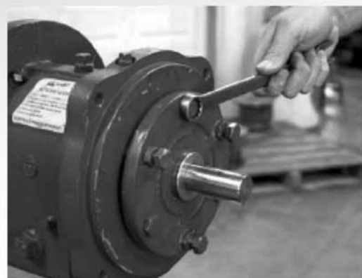
FIGURE 26 PRELIMINARY IMPELLER ADJUSTMENT
