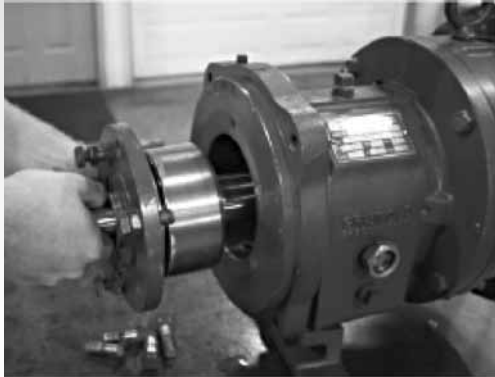
FIGURE 16 SHAFT/BEARING HOUSING REMOVAL
