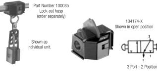
NOTE: ARO Safety Lock-out Valves meet OSHA Lock-out / Tag-out regulation 1910.147, which requires protection from unexpected start-up of a machine during service or maintenance.
