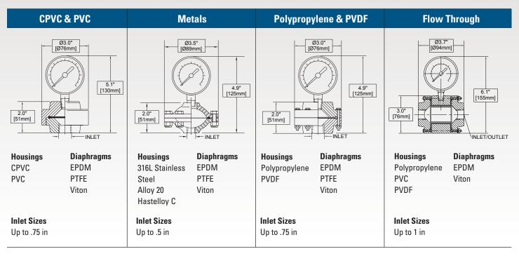
SENTINEL Diaphragm Seals, also referred to as 'gauge guards', employ a chemically resistant diaphragm to effectively isolate process fluids from gauges and other system instrumentation. The durable diaphragm allows SENTINEL to accurately transfer process pressure without direct contact with hazardous or corrosive process fluids.
