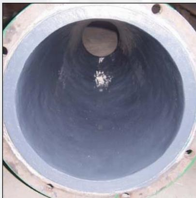
**Rubber linings** are typically undermined by glue failure at the seams, which can lead to catastrophic sheet delamination.
