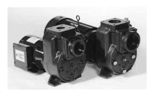
standard end suction centrifugal pumps the Griswold H Series is a true self-priming pump. Able to maintain it's prime even when check valves or foot valves have failed. The suction line being located higher on the pump housing than conventional centrifugal pumps keeps the impeller and mechanical seal covered with water at all times eliminating the need to re-prime the pump and protects the seal from running dry and costly replacements.
