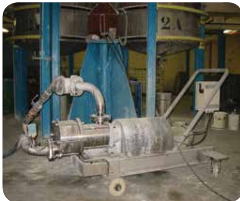
Mouvex C Series pump in paint filtration and conditioning.
