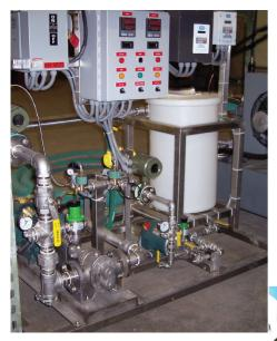
Utilizing ECO GA12 Flanged Pump to pump resin.
