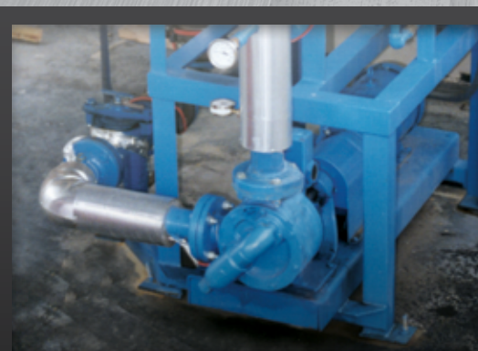
4925 series pump moving refrigeration ammonia.
