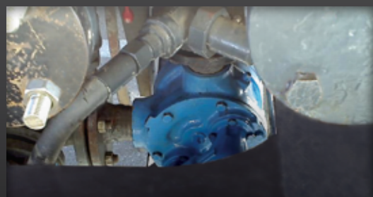
LP Gas pump moving LPG off of a truck.
