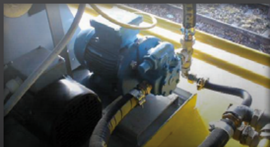
Flanged general purpose pump connected to flexible lines.
