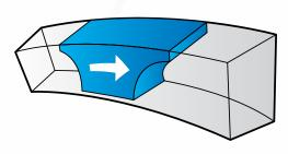
The deep channels in which the rotors travel provide large voids to minimize shear and bruising of solids.
